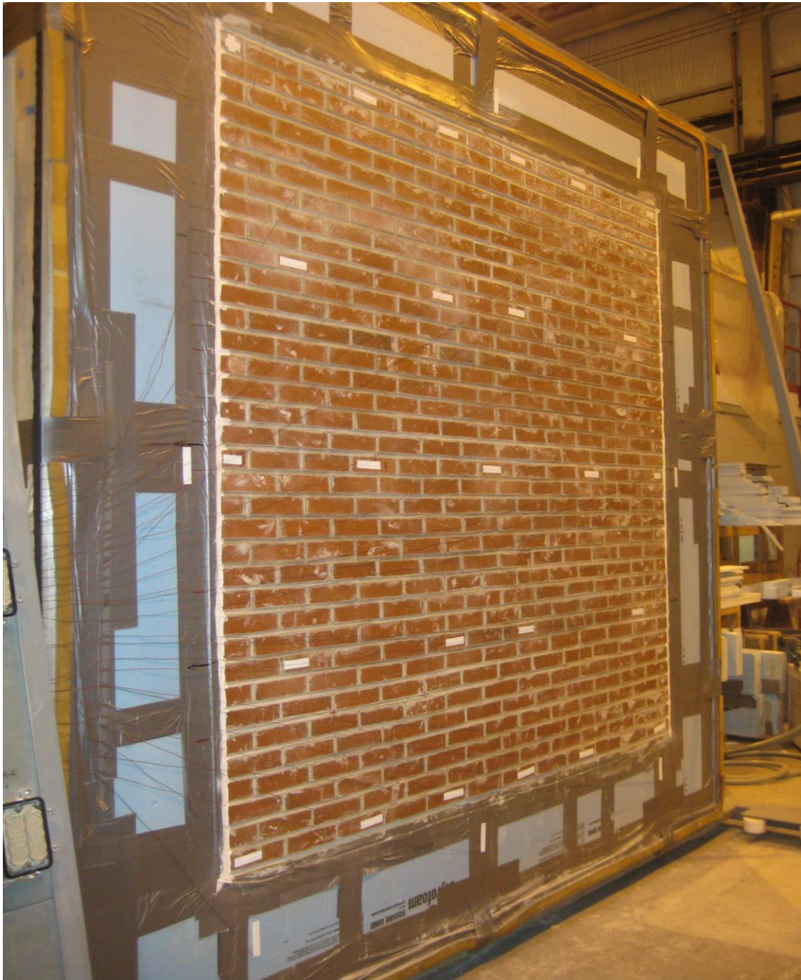
(Exterior Brick Wall Completed & Instrumented)
