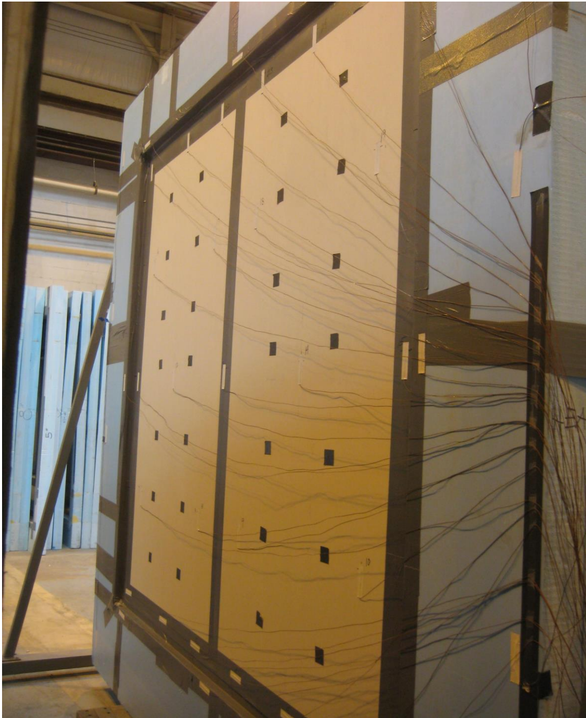
(Interior of Base Wall with Brick Ties Instrumented)
