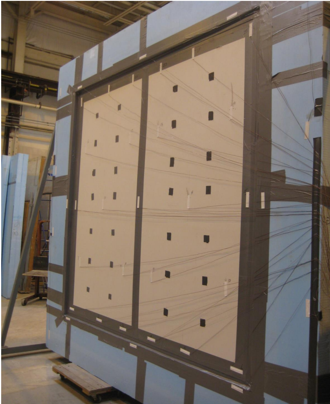
(Interior of Base Wall with-out Brick Ties Instrumented)
